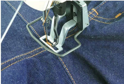
H, W type (Bartacking crotch of jeans)
