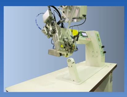
Hot air tape bonding uses extremely hot air to melt specialised welding tape ; the melted welding tape is then fused to the fabric as it passes through an upper and lower roller. The rollers apply pressure so the tape and fabric merge together.
