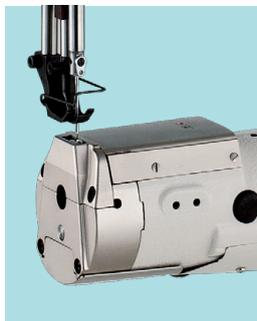
Thread tightness can be kept same, even the multi-level of material.
