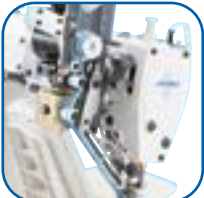
New type belt feed mechanism
