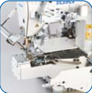
Electromagnetic needle thread / looper thread trimming device
