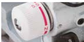
adjusts the lower knife quickly to change the width of fabric in the seam allowance, for perfect seams and rolled edges.
