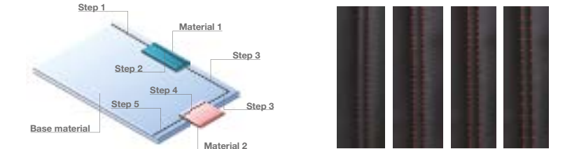
Example of design stitches by means of the custom pitch function
