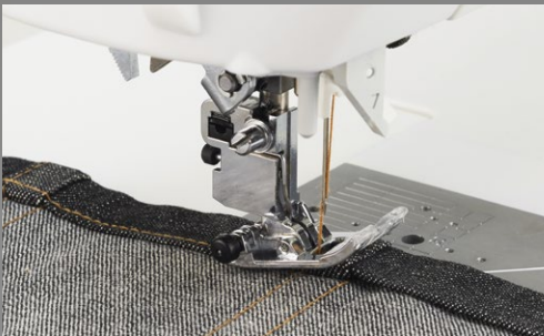
Sewing a flat fell seam on thick denim overlapped. Easily crosses seams of thick fabrics.
