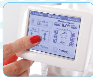
Programmable Needle up / down positions.
