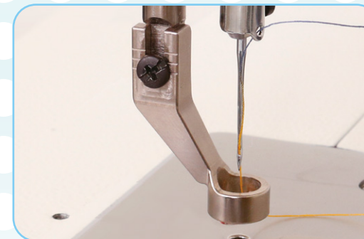
Quilting Foot Compatible with ¼ inch Long arm Rulers.
