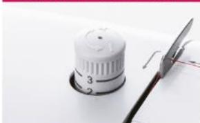
When sewing thin or thick fabrics, you can get comfortable feed.
