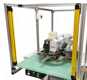
Machine Compact: 1.42 x 1.20m Safe: Safety light curtain
